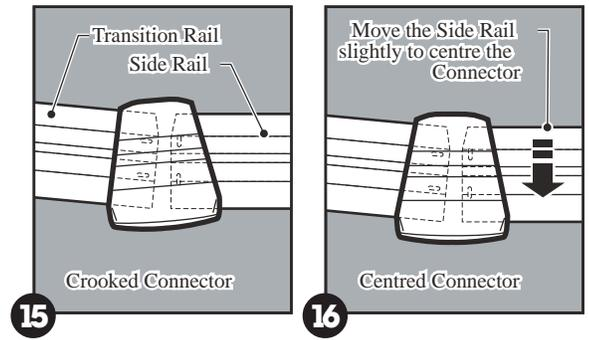
connector and loosen the screws on the side rail. Shift the side rail in or out from the centre of the pool until the connector can be properly centred between the rails (see diagram 16).
