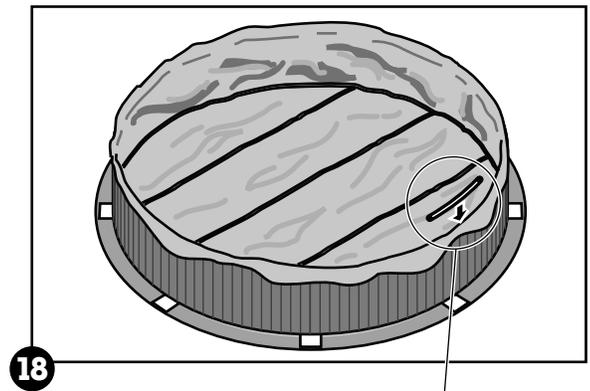
**2. Fasten the Liner in place (Overlap Liner only)**
