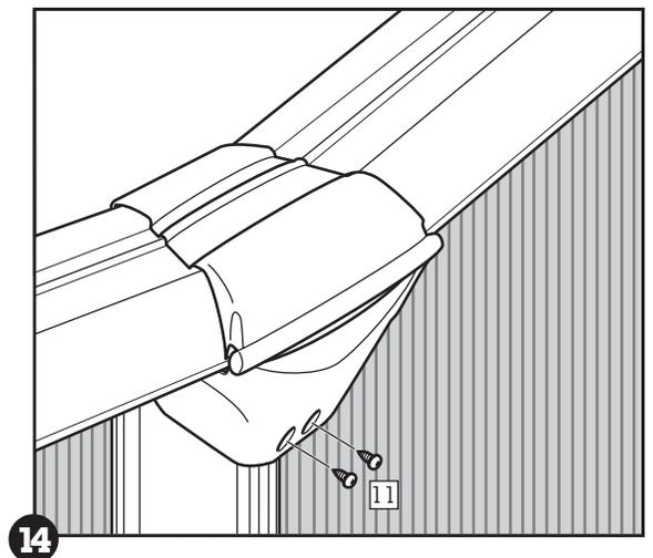
g. For oval pools only: at the transition points only, where the end rail meets the side rail, make sure the side rail lines up properly with the end rail. If it doesn't line up the connector will appear crooked from above (see diagram 15). If the connector isn't centred between the rails, temporarily remove the
