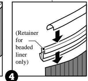
**Make sure** the gap is directly above the base plate (this applies to round pools, oval pools and Gibraltar Style pools). (If you have a **beaded pool liner**, set lengths of **liner retainer** on the top edge of the wall first, then the slotted tubes and connectors.)
