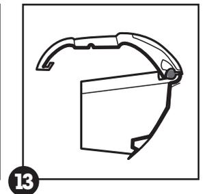
firmly in place. Bring the lower connector down into place under the top rails by spreading the sides out completely, as shown in diagram 11, and **gently** stretching it across and down, as shown in diagrams 12 and 13.
